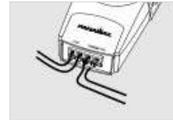
**STEP 3** Push the connector tab firmly away from yourself. The connector jaws will open. Push the stripped end of the wire into the connector. Repeat with the other three wires.
