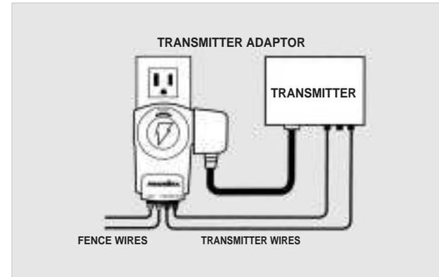
**STEP 1** Plug the lighting protector into a grounded (3-wire) 120V AC outlet within five feet of where you want to locate the transmitter
