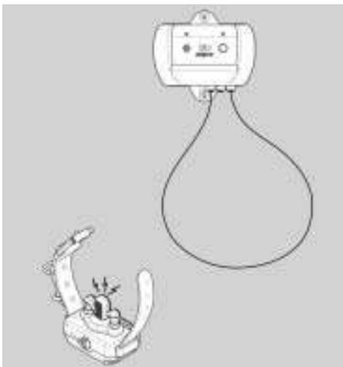
1. To ensure that your *dogtra* eF-3000 GOLD system is working properly, connect the transmitter adaptor into the adaptor of the transmitter and then plug the adaptor into a household outlet. Switch the stimulation knob to Pager+Stimulation, or Stimulation Only. The ON/OFF indicator light should turn on.
