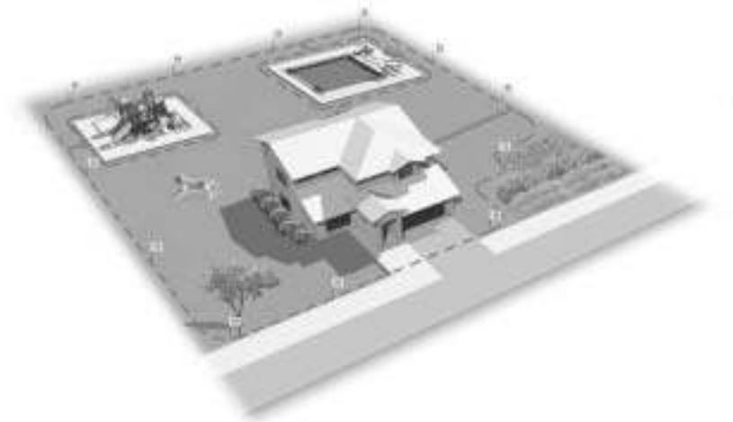
The fence wire must make a continuous loop around your property for your system to operate. The signal is delivered from the terminal of the transmitter, through the fence wire, back to the other terminal on the transmitter. When this is accomplished, the wire continuity light will emit a constant red indicator.
